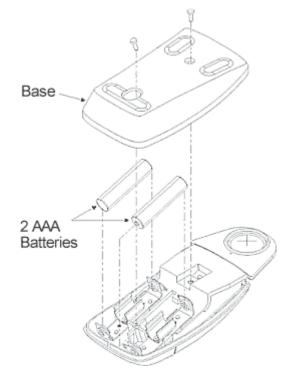
When you replace the cordless cursor batteries, the cursor will reset to the default frequency. If you changed the frequency of the cursor before replacing the batteries, you will need to do so again after replacing the batteries (see the *Reducing Monitor Interference* section in the *Troubleshooting Guide*).
