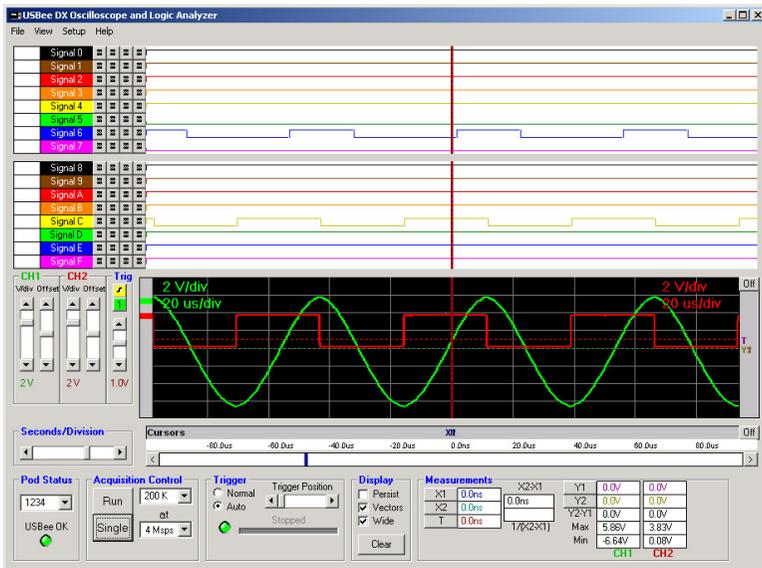
The USBee DX Mixed Signal Oscilloscope functions as a standard Digital Storage Oscilloscope combined with a Digital Logic Analyzer, which is a tool used to measure and display analog and digital signals in a graphical format. It displays what the analog and digital input signals do over time. The digital and analog samples are taken at the same time and can be used to debug mixed signal systems.
