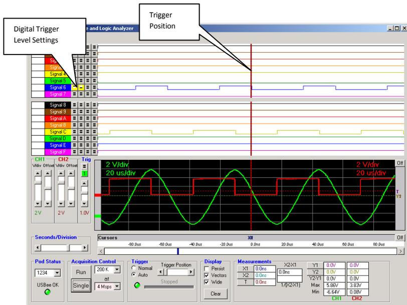
The digital trigger condition is made up of up to 4 sequential states of any of the 16 signals. Each state for a single signal can be high, low or don't care. This allows you to trigger on rising edges, falling edges, edges during another signals constant level, or one edge followed by another edge.
