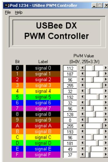
Each channel outputs a repeating waveform with a 1kHz frequency. The period of the repeating waveform is made up of a high duration followed by a low duration and has 256 steps. The length of the High duration is the PWM value that is shown. The length of the Low duration is 256 – the High duration.
