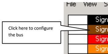
To setup a single line on the waveform display as a bus, click on the white box to the left of the signal name. The Channel Settings dialog box will appear as below.
