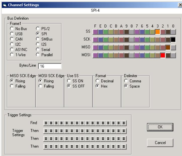
On the above dialog box, select the signals you plan to use for the SPI protocol. Also set the appropriate sampling edges for both data lines and if you would like to use the SS (slave select) signal. If you turn off the SS, all clocks are considered valid data bits starting at the first clock detected. Also choose what output format you want the traffic.
