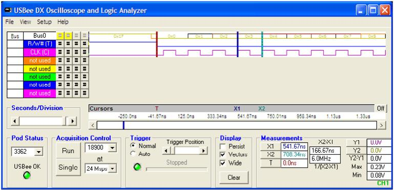
As a comparison between the modes, all transfers in high speed mode (all 160,000 samples) occur before the first dark blue cursor on the logic analyzer trace below. The Bi-Directional writes from the SetSignals (16000 samples) occur between the cursors, and the bi-direction reads occur after the second cursor.
