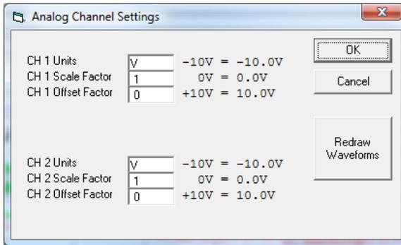
Below shows a setting of mA with various gains and offsets. Instead of displaying the actual value measured in volts, the display will show the scaled value in the new units.
