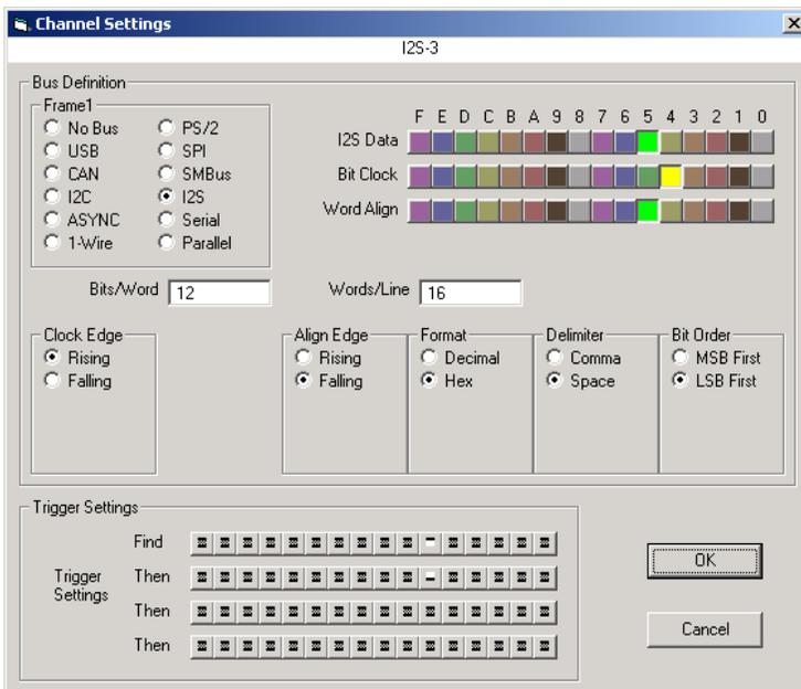
On the above dialog box, select the signals you plan to use for the I2S Bus protocol. Select the start edge for the external word align signal, the Bits/Word and the Clock sampling edge. Choose the bit ordering as well as the output format of the traffic.
