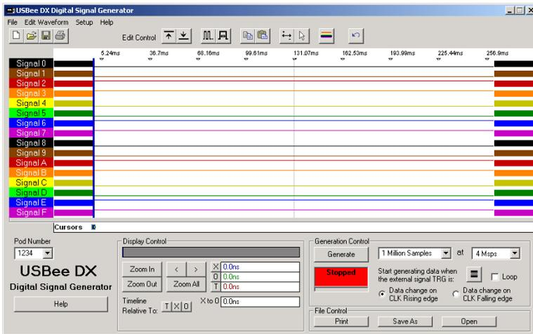
The Digital Signal Generator is used to actively drive the 16 digital signals with a voltage pattern that you define.
