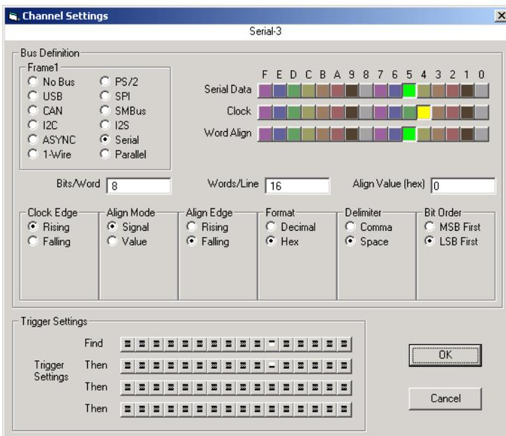
On the above dialog box, select the signals you plan to use for the Serial Bus protocol. Select whether you have an external word align signal (Align Mode = Signal) or if your serial data has an embedded sync word in the data stream (Align Mode = Value). The Bits/Word is the size of the Sync word as well as the output word size. Choose the bit ordering as well as the output format of the traffic.
