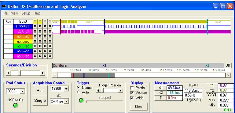
The following traces show the low level timing for the Bi-Directional Mode SetSignal and GetSignal calls.
