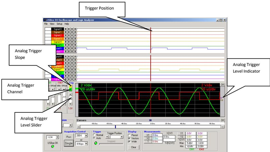
For an **Analog trigger**, you can specify the trigger voltage level (-10V to +10V) by using the slider on the left hand side of the analog waveform display. A red line that indicates the trigger level will momentarily be shown as you scroll this level. A small T will also be shown on the right hand side of the screen (in the cursors bar) that shows where this level is set to.
