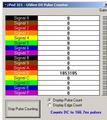
To start counting the pulses or edges on the signals press the Start Puls Counting button. The pulses are counted and the current range of pulses is displayed. In this case the system is counting all pulses down to 166.7nsec wide.
