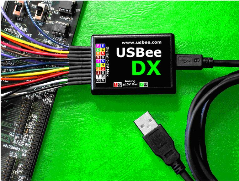
The USBee DX Test Pod is a large sample buffer PC and USB based programmable multifunction digital storage 2-channel oscilloscope, 16-channel logic analyzer and digital signal generator in a single compact and easy to use device. It is the ideal bench tool for engineers, hobbyists and students
