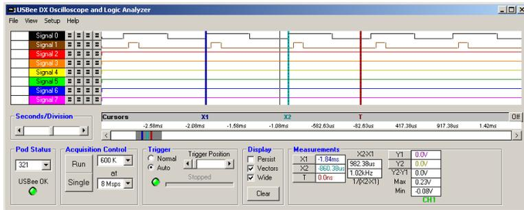
The above shows 2 outputs of the PWM Controller. Signal 1 shows the PWM value set to 31 (out of 255) and Signal 0 shows the PWM value of 137. A value of 0 is all low, and a value of 255 is mostly high (one out of 256 is low).
