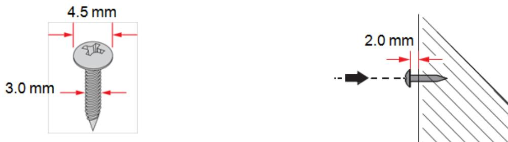
Figure 10: Securing Wall Mounting Screws
