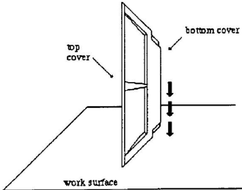
5. Lay the tablet right-side-up on the work surface. Grasp the tablet edge that you just loosened in Step 4. With your thumbs on the top cover and your finger tips on the edge of the top cover, pull the top cover up until the tabs snap loose.
