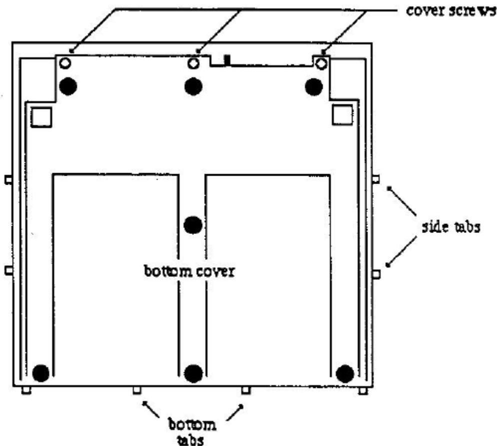
Notice the bottom and top covers are held together by tabs on the bottom cover.
