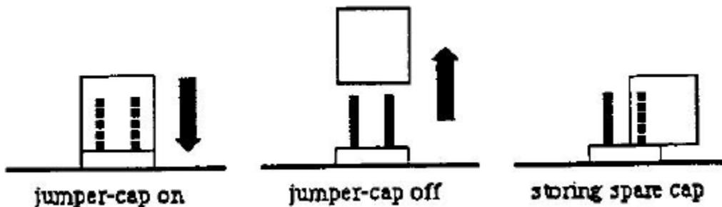
Hint: A cap is "attached" when it straddles both pins. It is "removed" when it is on no pins or on only one pin. Therefore, a handy way of storing a spare cap is to stick it on only one jumper pin.
