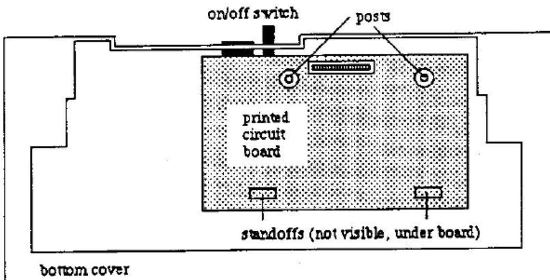
The board should slip into this position very easily. If at any time you feel that you had to force it, then it is not seated properly. Wiggle the board until it drops easily onto the standoffs.
