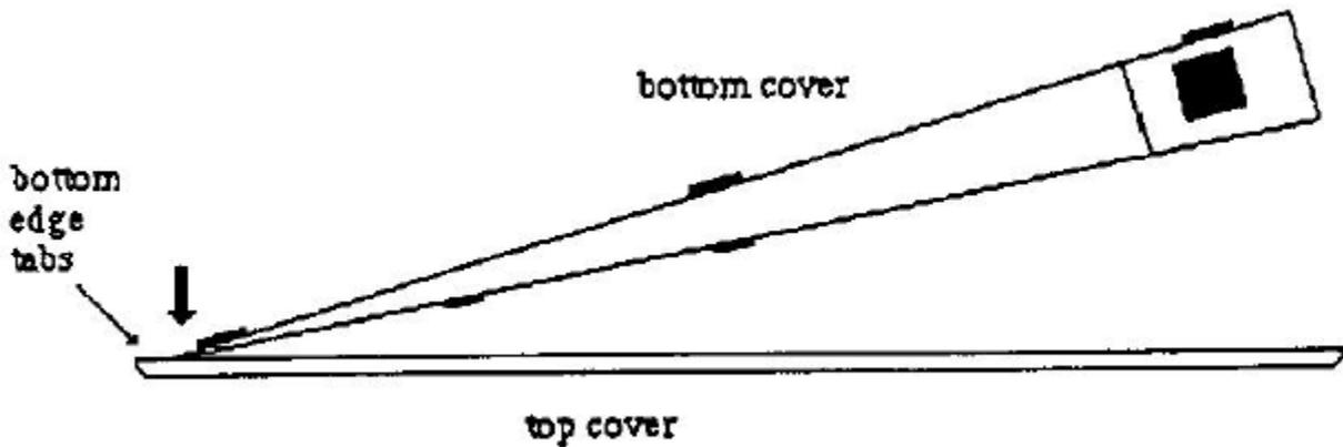
5. Snap the bottom cover down against the top cover. The bottom and side tabs should be seated in the slots.
