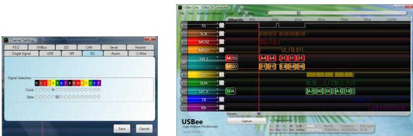
We then add the Async bus using the Channel Settings dialog box as below with the resulting waveline.
