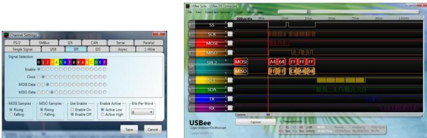
From here we select the parameters for this bus (shown above) and press Save. Once we press Save, the line is added to the screen, the current trace is decoded, and the decoded information is shown on the waveline.
