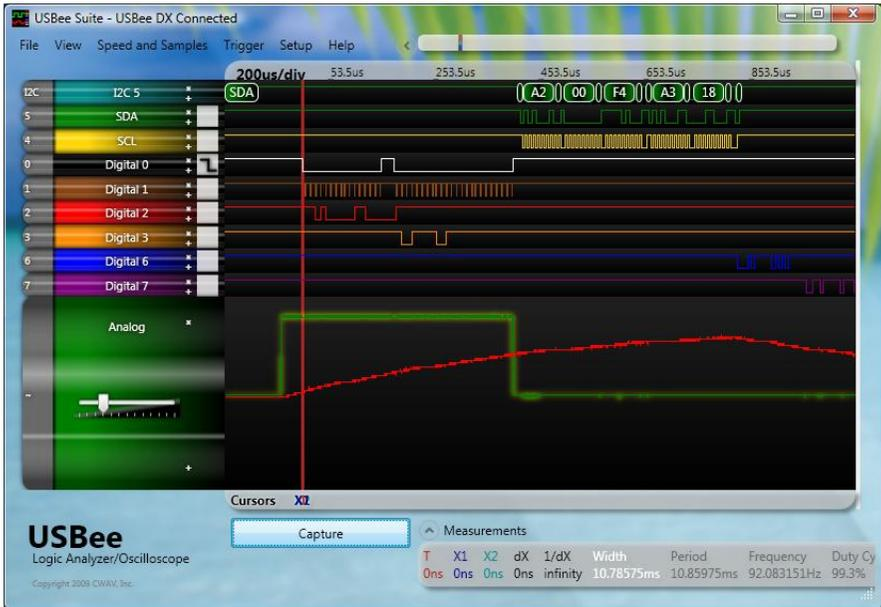
The **Quick Setup – ASYNC** configures the signals 6 and 7 to be a full duplex ASYNC bus with the TX and RX lines. You will need to change the baud rate, data bits and parity to match your bus. It also adds a decoder line to the screen with this data decoded as below.
