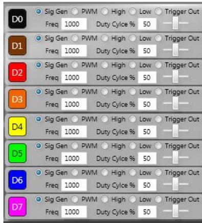
Each of the 8 digital lines can have one of 5 different modes by selecting the associated radio button above:
