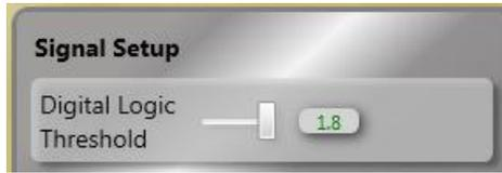
The USBee RX features variable Digital Logic Thresholds that can range from -1V to +2V. Set this logic threshold to define the voltage level that indicates the change from a logic "0" to a logic "1".
