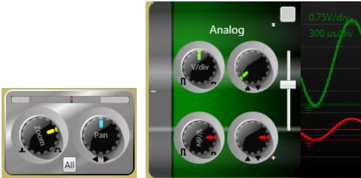
To **Scroll the Waveforms in Time** left and right, you can click on the overview bar above the knobs, scroll the **Pan knob** (click and drag or mouse wheel on the knob) or you can simply click and drag the waveform itself with the left mouse button.
