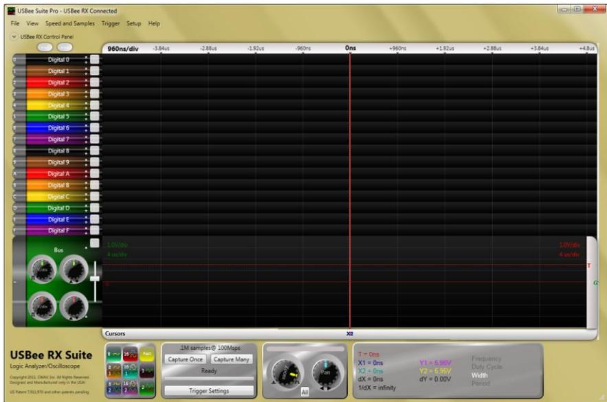
The USBee RX Suite maintains its last configuration and will reload that configuration when it is run again. This configuration is located in your `\Users\NAME\AppData\Local\USBeeSuite` directory where NAME is your username. To reset the software to the initial state you can delete the files in that directory.
