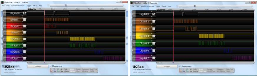
Removing a signal from the screen may not remove the signal from subsequent captures. Signals will only be eliminated from captures if all signals from a given byte lane are removed.
