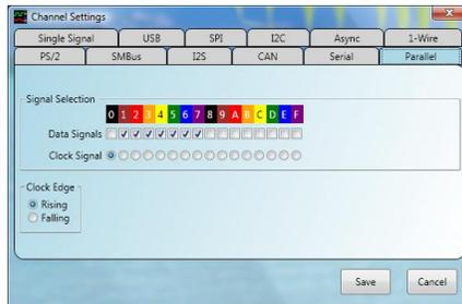
On the above dialog box, select the channels you want to include in the parallel data bus. You can also use any one of the 16 digital signals as an external clock. Choose if you want to use the external clock signal and the external clock edge polarity.
