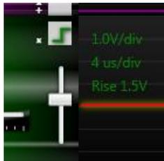
For an analog trigger, the trigger position is where the waveform crossed the **Trigger Voltage** level that you have set at the specified slope. To move the trigger voltage level, just move the slider on the left of the waveform.
