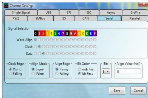
On the above dialog box, select the signals you plan to use for the Serial Bus protocol. Select whether you have an external word align signal (Align Mode = Signal) or if your serial data has an embedded sync word in the data stream (Align Mode = Value). The Bits/Word is the size of the Sync word as well as the output word size. Choose the bit ordering as well as the output format of the traffic.
