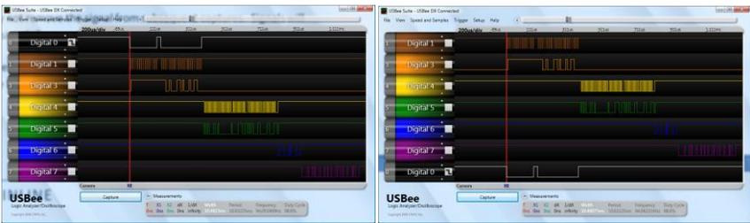
To **Add a Waveline**, click on the small + sign above where you want to insert the new waveline. Below you see a new waveline inserted after the first waveline.
