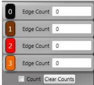
Counting occurs when the **Count** checkbox is selected. To clear the counts, press the **Clear Counts** button. Remember that the counts are affected by the **Digital Logic Threshold** setting, so you must set this correctly for the signals you are measuring for accurate counts.
