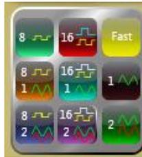
The **FAST** button sets the Sample Rate and buffer size to give the fastest screen update rates.
