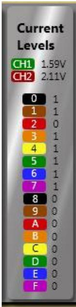
The USBee RX constantly monitors the state of all of the digital inputs and the voltage levels of the CH1 and CH2 inputs. This way you can see the state of the channels even at times you are not capturing waveforms using the Mixed Signal Oscilloscope.
