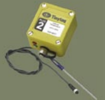
Place Data Logger in position to record and connect probe if required
